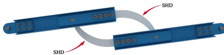
Fig. 1 Design concept of the proposed brace member
